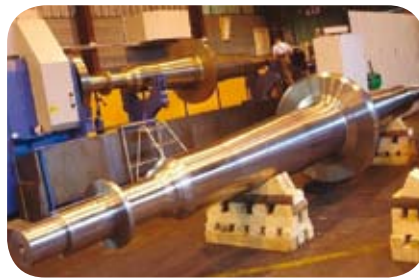
Clockwise from left: kiln support rollers at SFAR ready for shipping Alternator shaft on milling machine Fan shaft on parallel lathe Motor shaft on grinding machine
