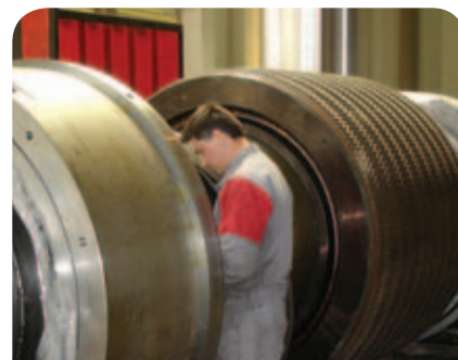
SfarSteel offers finished forged rollers for roller presses, incorporating three layers of niobium carbide, deposited by submerged arc techniques. Sizes range up to 3m in diameter and weigh up to 60t
